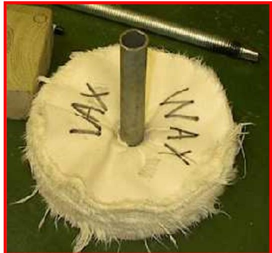
4. Here you see the punch all the way through the cloth wheel with the punched out cotton holes inside the conduit. This must be done with all three of the wheels before going on to the next step. You see the white diamond wheel with the punch sticking out one side and the Tripoli with the punched out linen, flannel & cotton holes scattered around. Making certain that your punch is very sharp is the key.
