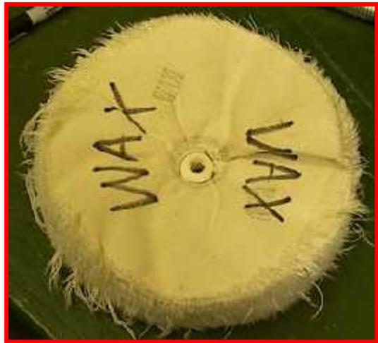
3. I made a punch from a piece of 3/4" electrical conduit. Cut the conduit to 6" length and grind one end to make it sharp. You need a block of end grain wood to pound on when punching out the 3/4" hole. Keep rotating the punch as you hit the end with as large a hammer as you have (I used a small sledge) until the punch goes all the way through the cloth wheel.
