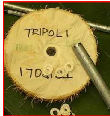
5. Once the 3/4" holes are punched in the cloth wheels, it's time to make 3/4" inserts from 3/4" copper water pipe. Using a copper pipe cutter, make three inserts for the wheels and make certain that they are 3/8" in length, but no longer. They will keep the wheels centered on the shaft but must not be as wide as the cloth wheels are thick. The large washers & nuts will clamp the wheels to the shaft.
