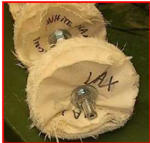
8. This photo shows the lathe drill chuck attached to the opposite end of the shaft. Note the large washers and nuts on each side of each wheel holding each wheel tightly to the shaft. Each end of the shaft has a 3/4" lock washer to keep everything in place. The spacers are tight between the nuts but not overly tight. They cannot turn on the shaft and keep those revolving threads away from errant fingers.
