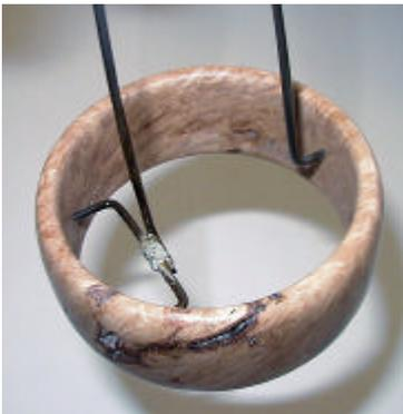
**Put on one or two coats of sanding sealer and hand sand. With a 3 prong spring holder I spray 2 to 3 coats of lacquer.**
