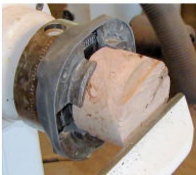
**True up the face of the block to the desired width, marking the center with an indentation.**
