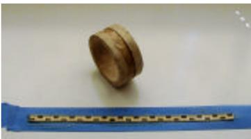
**Stick the inlay strip to 2 or 3 layers of masking tape. Apply contact to the strip and the groove on the bracelet blank.**
