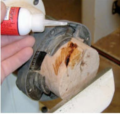
**Fill any cracks or voids with CA glue.**
