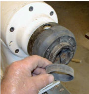
**A piece of a small tire tube is cut and put over the jaws of the chuck to protect the inside of the bracelet. Note: I also use a larger piece to protect my hands and tools from the chuck.**
