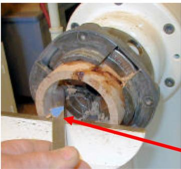
**With a 3/8" round nose scraper clean up the inside. Tilt the tool handle down to give a shear scraping cut. Turn blank around and clean the other half. The blue tape is a depth gage so I don't go in to far.**
