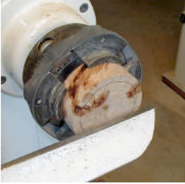
**Turn the blank around and repeat. True up the face, mark center and mark the parting line.**
