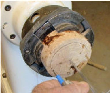
**With a compass set to  $\frac{1}{2}$  the inside diameter draw a line to mark for the parting tool.**
