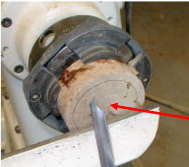
**Use a narrow parting tool that has a modified tip.**
