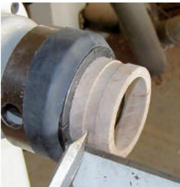
**Remove the wood to the depth of the inlay with a standard parting tool.**
