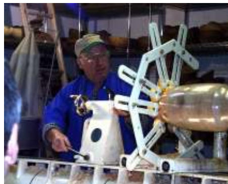
Gary bores a hole prior to hollowing a vase. Note the shop-built steady rest
