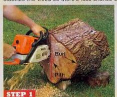
Chainsaw through the pith of the oversize section to remove the back half of the log while also flattening the back of the burl.
