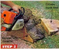
Trim the excess trunk ends, then chainsaw along the sides of the burl to square it, as shown here.
