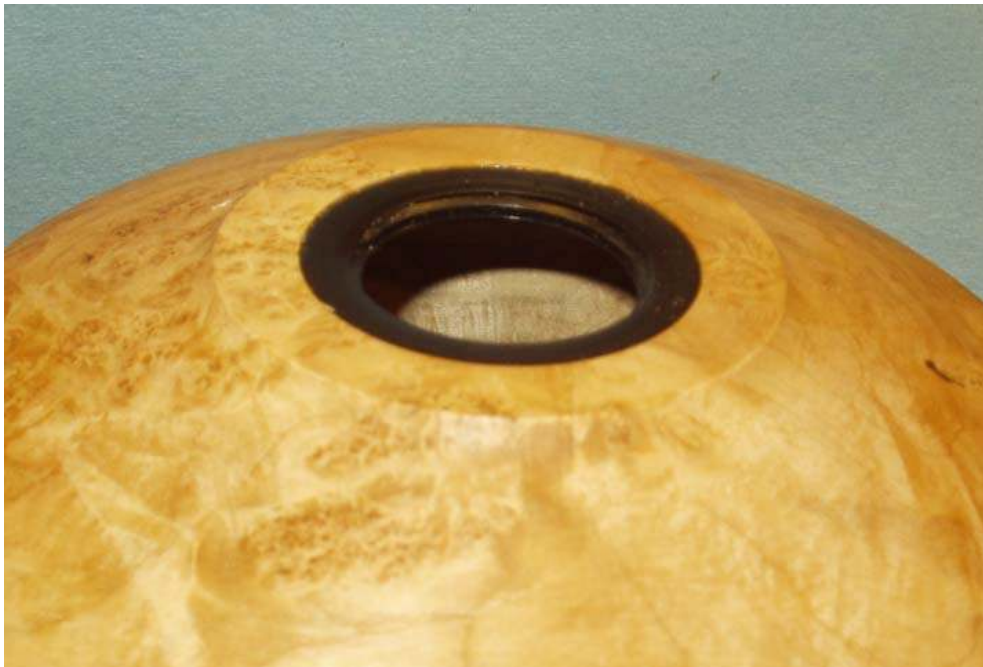
Here are the female threads glued into the neck of the urn.
