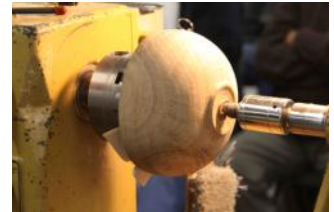
Tom turning the foot of the bowl on a jam chuck.
