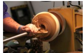
Hollowing a vessel with a captured hollowing system.
