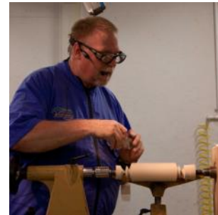
Tom uses a jig to mount his router, 60 degree cutter, and a Baxter Threading Master.
