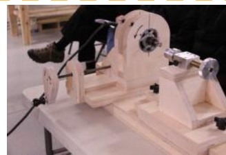
Tom uses a jig to mount his router, 60 degree cutter, and a Baxter Threading Master.
