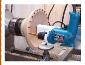
Drilling the 24 equally-spaced holes with the Oneway Drill Wizard and my 3/8" drive drill motor that had to be purchased to fit the collar of the Drill Wizard.
