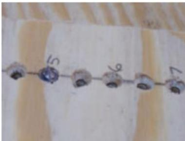
I made two different pivot pins: one shown in the five inch position in the above photo; the other was a bit longer for thicker blocks of wood. I used the short one to cut flat boards and the longer one to cut half log sections as shown below.
