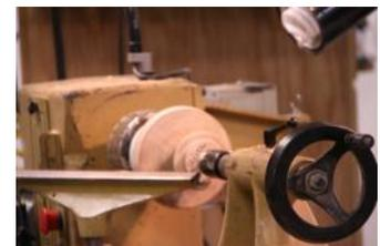
Mounting the sanding mandrel in the headstock allows you to sand the wings of the bowl.
