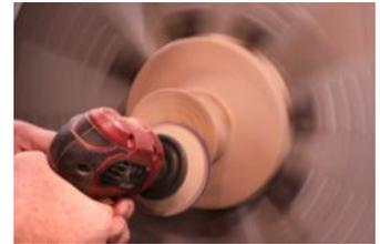
When using Cole jaws keep the RPMs below 1000.
