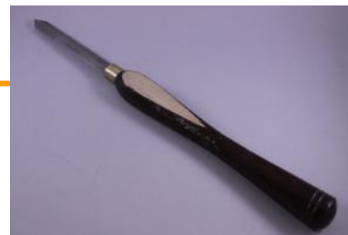
Making a flat spot on the tool handle will stop the tool from rolling off of the lathe bed or work table.
