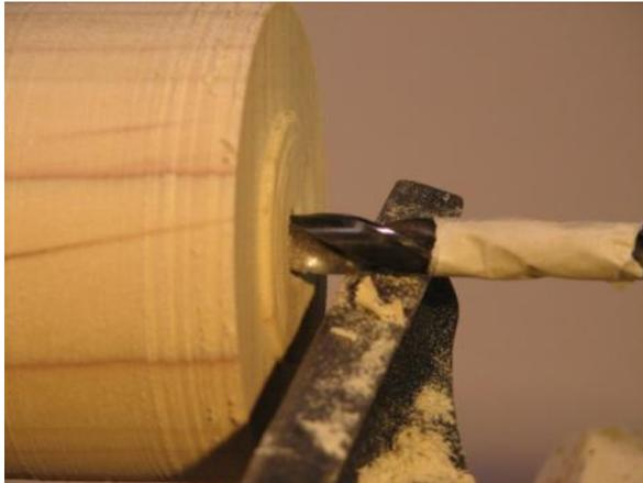
**Drilling a pilot hole in the end of the blank to simplify hollowing and to establish a depth for the bottom of the bowl.**
