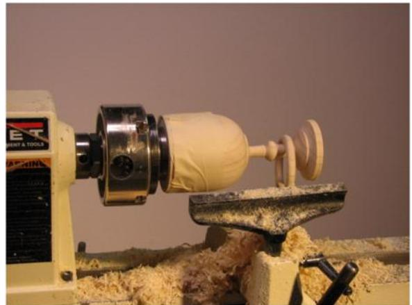
Use the live center in the tail stock to add additional support while the bottom of the goblet foot is finished. Remove the tail stock to finish the middle of the base.
