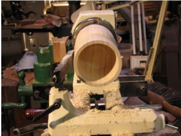
**Sand the goblet bowl and apply finish if you are using a lathe applied product.**
