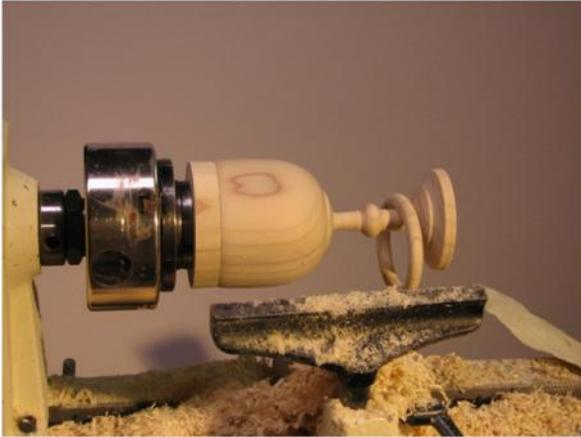
**Turn a spigot on the waste block so that the mouth of the goblet is a snug fit on it.**
